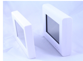
The MiniTouch 1/2 as thick and much smaller than the SuiteTouch while maintaining a 5" display
